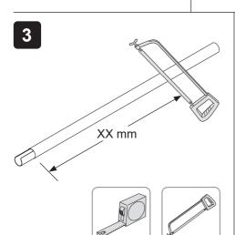
Cut to length using a hack saw. **Ensure parts are fully de-burred.**
