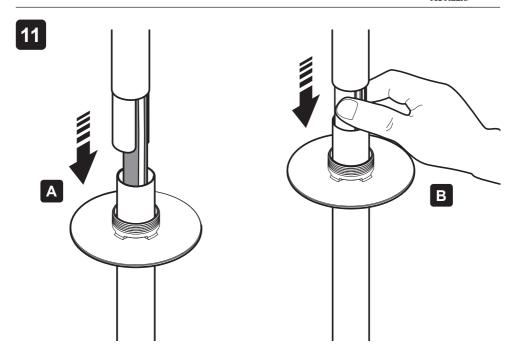
Squeeze together the end of the joiner section of the extension riser so that it can be pushed in the top of the main riser.
